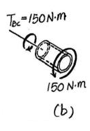
•5–77. The A-36 steel shaft has a diameter of 50 mm and is fixed at its ends A and B. If it is subjected to the torque, determine the maximum shear stress in regions AC and CB of the shaft.
