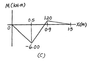
6–103. Determine the largest uniform distributed load w that can be supported so that the bending stress in the beam does not exceed  $\sigma_{\rm allow}=5~{\rm MPa}$ .
