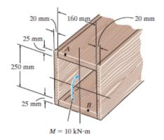
The moment of inertia of the cross-section about the neutral axis is
