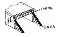
6–62. A box beam is constructed from four pieces of wood, glued together as shown. If the moment acting on the cross section is  $10 \text{ kN} \cdot \text{m}$ , determine the stress at points A and B and show the results acting on volume elements located at these points.
