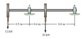
The FBD of the shaft is shown in Fig. a
