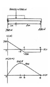
**6–91.** Determine the absolute maximum bending stress in the 80-mm-diameter shaft which is subjected to the concentrated forces. The journal bearings at A and B only support vertical forces.
