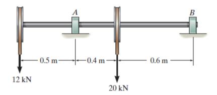
6- The two solid steel rods are bolted together along their length and support the loading shown. Assume the support at A is a pin and B is a roller. Determine the required diameter d of each of the rods if the allowable bending stress is  $\sigma_{all}$  = 130 MPa.
