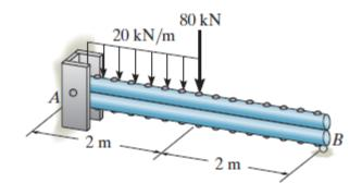
7- Determine the largest uniform distributed load w that can be supported so that the bending stress in the beam does not exceed  $\sigma_{all}$  = 5 MPa.
